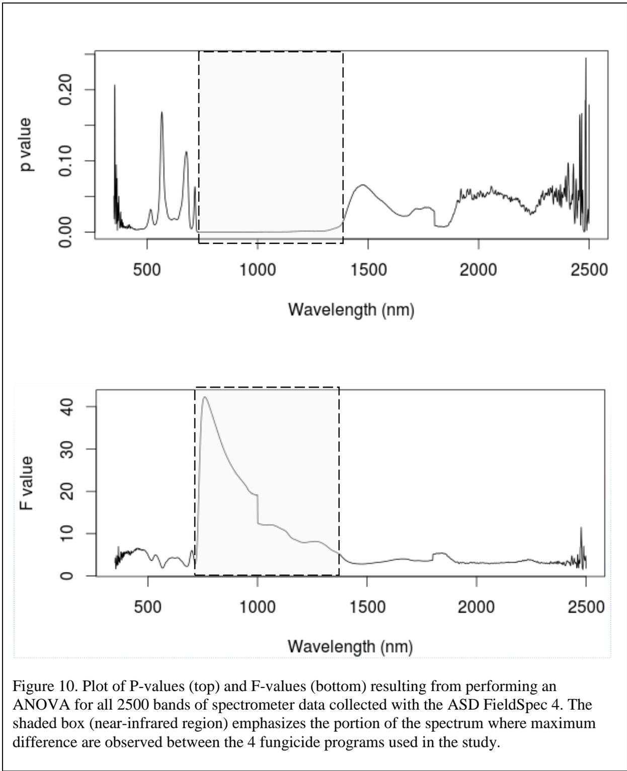
Figure 10. Plot of P-values (top) and F-values (bottom) resulting from performing an ANOVA for all 2500 bands of spectrometer data collected with the ASD FieldSpec 4. The shaded box (near-infrared region) emphasizes the portion of the spectrum where maximum difference are observed between the 4 fungicide programs used in the study.
